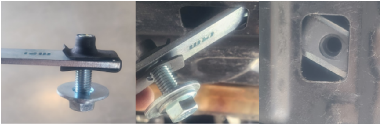
1: Partially thread bolt.
