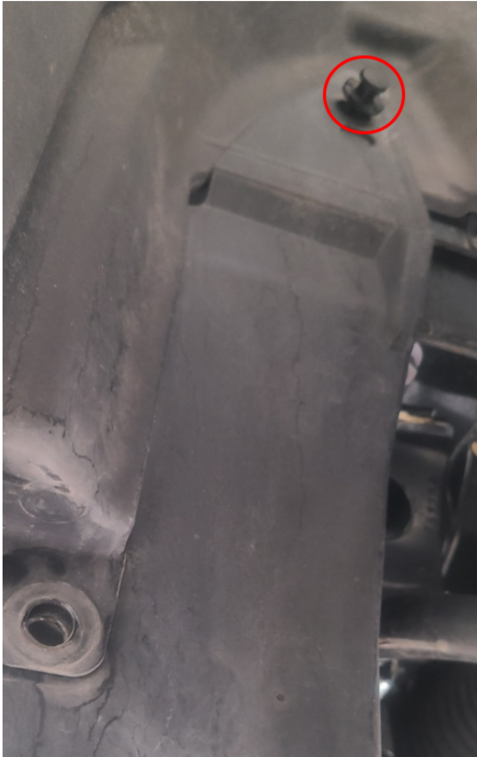
Figure #: Upper Side View of Retaining Clips to Remove
