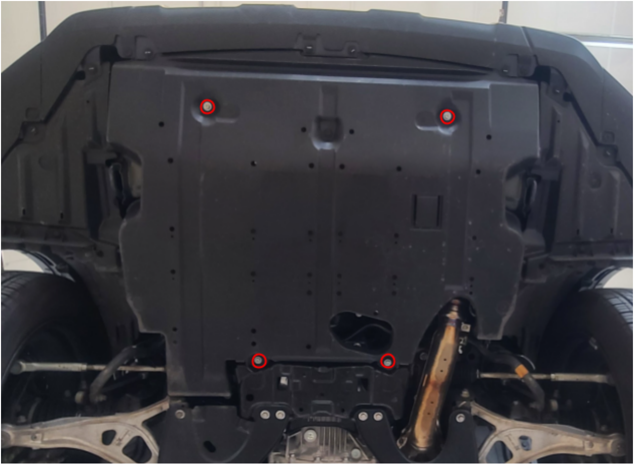
Figure #: Bottom View of Bolts to Remove
