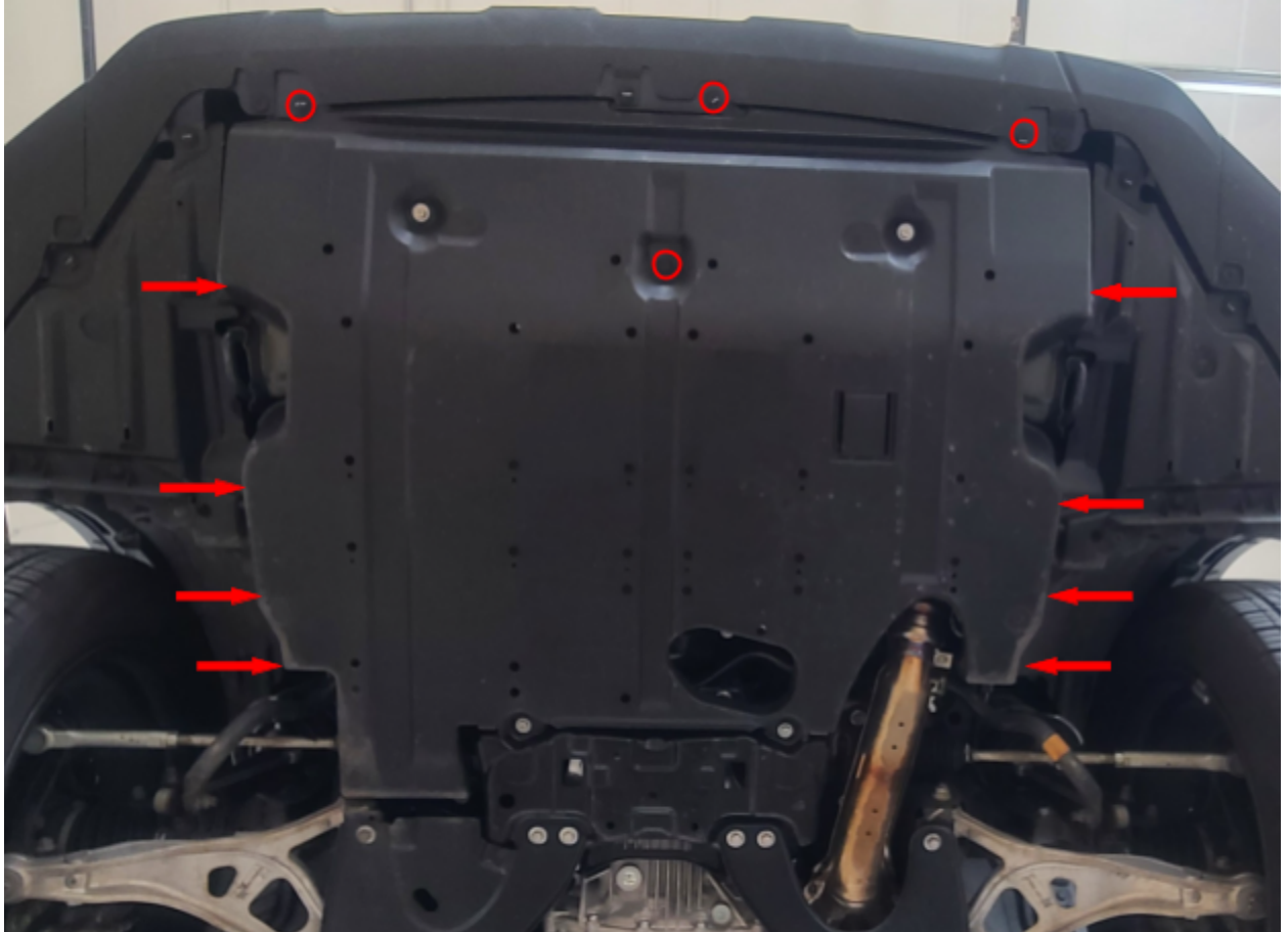
Figure #: Bottom View of Plastic Clips to Remove
