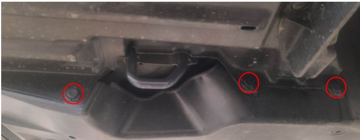
Figure #: Lower Side View of Retaining Clips to Remove
